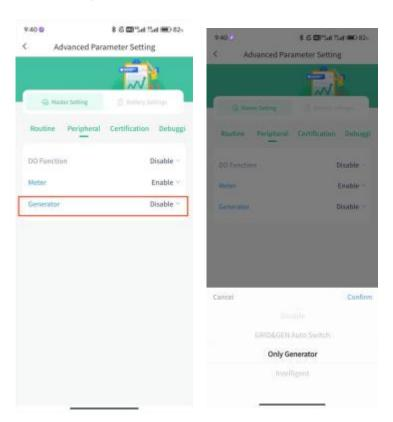
When there is no ATS and the oil generator is directly connected to the inverter grid port, this option needs to be selected. The relevant
