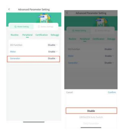
In addition to the above two modes, there is also a disable option. In this mode, the inverter defaults to the grid access mode.
