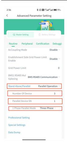
The number of device is set to 3, the is set to 1, 2, and 3(Corresponding to the three phases A, B and C, 1 corresponds to phase A, 2 corresponds to phase B, and 3 corresponds to phase C), and 1 phase parallel mode is set to three-phase
