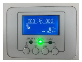
The user can enter the parameter setting **page 12** of the screen to modify the password, as shown above. The password modification
