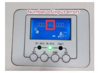
After long pressing the "ENT" key to confirm the password, if the password is correct, you can enter the parameter setting page. If the password is wrong, you need to re-enter the password for a total of **5 times**. At this time, the middle page number is displayed as the number of incorrect password inputs, as shown above. After five cumulative incorrect inputs, you need to wait **5 minutes** and try again.
