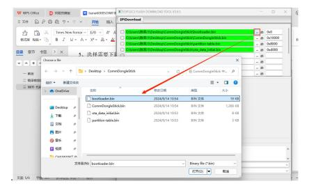
6.Check the file, set the corresponding addresses of the 4 burning files (note that the files and addresses must correspond one to one); select the Com port (depending on the computer port connected to the USB), set the baud rate to 460800; select 80MHz for SPI Speed.
