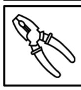
Crimping pliers: Crimp PV, BAT cable wires.
