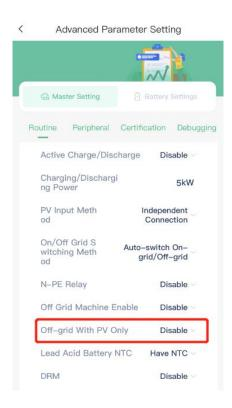
Note: When this function is enabled, the inverter is not connected to the grid or battery, and the PV can supply power to the load alone. If this function is not enabled, the inverter is not connected to the grid or battery, and the PV will not supply power to the load alone.
