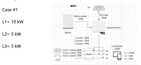
In off-grid mode, the isuna inverter can support 100% three-phase unbalance, that
