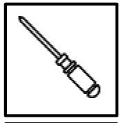
M6 screwdriver: Removal and installation of screws and wiring.
