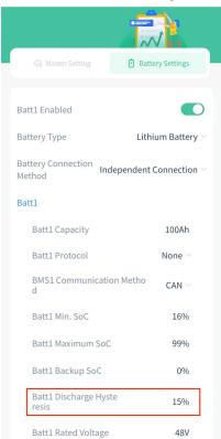
The above four settings are all for lithium battery SOC and are not effective for lead-acid batteries and supercapacitors.
