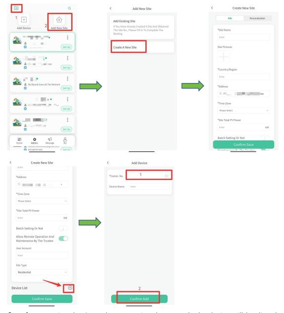
After scanning the QR code or entering the PN code, the device will be directly bound. Then return to "Admin." -> "Set Up" -> "Network Distribution" for distribution network.
