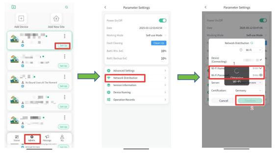
2. Select the inverter code to be assigned in "Admin." and assign it to the end user's account (one device is only allowed to be bound to one end user's account).
