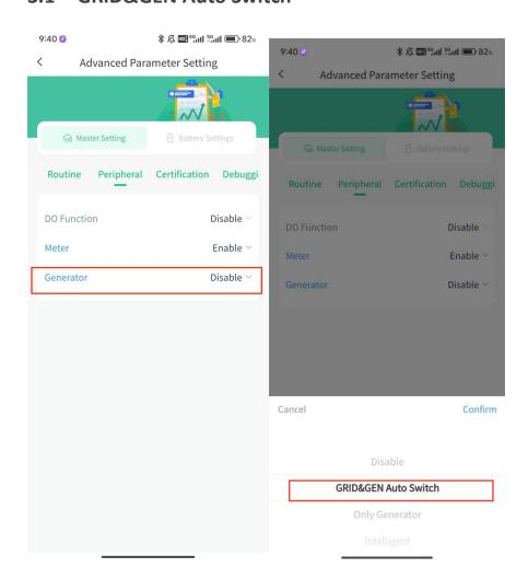
Note: The GRID&GEN Auto Switch needs to be used with an external ATS.
