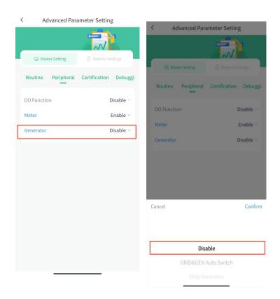
In addition to the above two modes, there is also a disable option. In this mode, the inverter defaults to the grid access mode.
