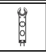
Removal tool: Remove and install the PV terminal.
