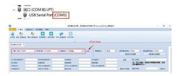
3. If the connection is successful, click the position shown in the figure below. The inverter operation status will be displayed; if not, you need to check whether the above steps are correct.
