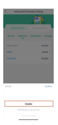
In addition to the above two modes, there is also a disable option. In this mode, the inverter defaults to the grid access mode.
