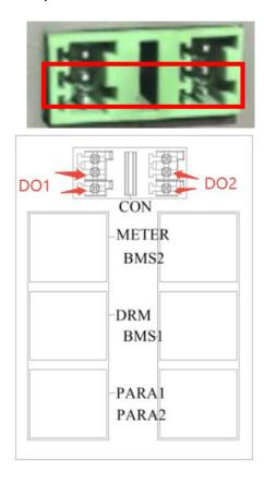
**Note**: The inverter has two DO ports for generator control: left side is The DO port DO1 of the GEN control corresponds to the lower pins of PIN1 and PIN2 as shown in the figure. When the inverter needs to control the GEN to start, the relay connected to DO1 closes, and the PIN1 and PIN2 pins are conductive. When the inverter needs to control the GEN to stop, the relay connected to DO1 opens, and the PIN1 and PIN2 pins are not conductive.
