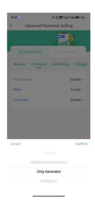
When there is no ATS and the oil generator is directly connected to the inverter grid port, this option needs to be selected. The relevant
