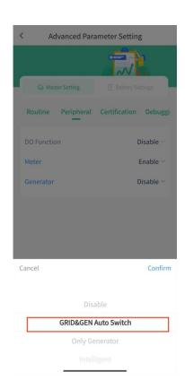
Note: The GRID&GEN Auto Switch needs to be used with an external ATS.
