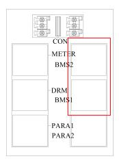
Connect the EMS to either BMS1 or BMS2. Let take BMS1 as an example. This interface is a multiplexed interface, where pin 1 and pin 2 are used to communicate with external EMS device, as shown below:
