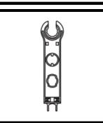
Removal tool: Remove and install the PV terminal.
